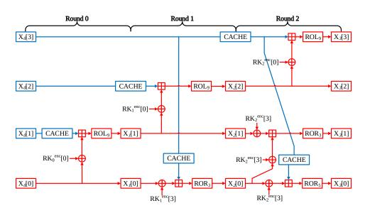
Figure 7. Optimized three rounds of LEA-128/128 block ciphers.
