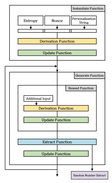
Figure 3. Detailed procedures of CTR\_DRBG [6,7].
