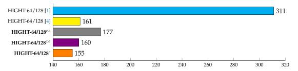
**Figure 13.** Comparison of execution time for HIGHT implementations on 8-Bit AVR Microcontrollers under the variable-key scenario in terms of clock cycles per byte, *c*: counter mode of operation (32-bit counter), *s*: building precomputation table separately from encryption process, *o*: building precomputation table online while executing the encryption process.
