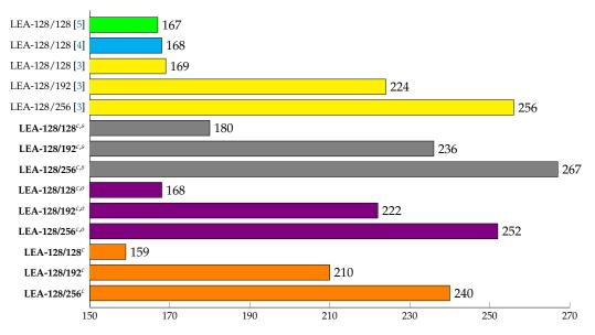
**Figure 12.** Comparison of execution time for LEA implementations on 8-Bit AVR Microcontrollers under the variable-key scenario in terms of clock cycles per byte, *c*: counter mode of operation (32-bit counter), *s*: building precomputation table separately from encryption process, *o*: building precomputation table in online while executing encryption process.
