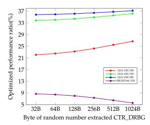
**Figure 14.** Performance improvement ratio (%) for CTR\_DRBG using our LEA and HIGHT implementations on 8-bit AVR MCUs, compared to CTR\_DRBG using previous LEA and HIGHT implementation [3–5]. The result is based on the number of extracted random numbers. B represents byte.
