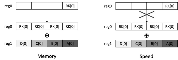
Fig. 9. Memory Optimization AddroundKey(Left) and Speed Optimization AddroundKey(Right)
