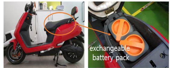
Fig. 10 Prototype of electric motorcycle installed exchangeable battery pack
