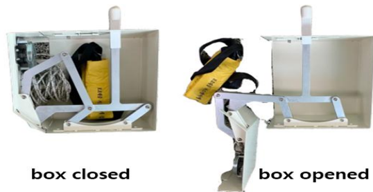
Fig. 10 Operating process for one-touch escape
