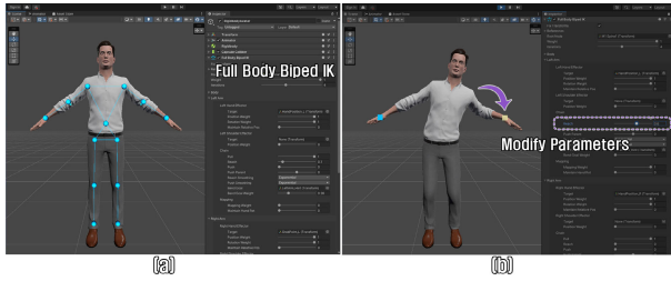
FIGURE 4. Example of virtual avatar joint movement according to the Full body biped IK component in the final IK and adjusting parameters.
