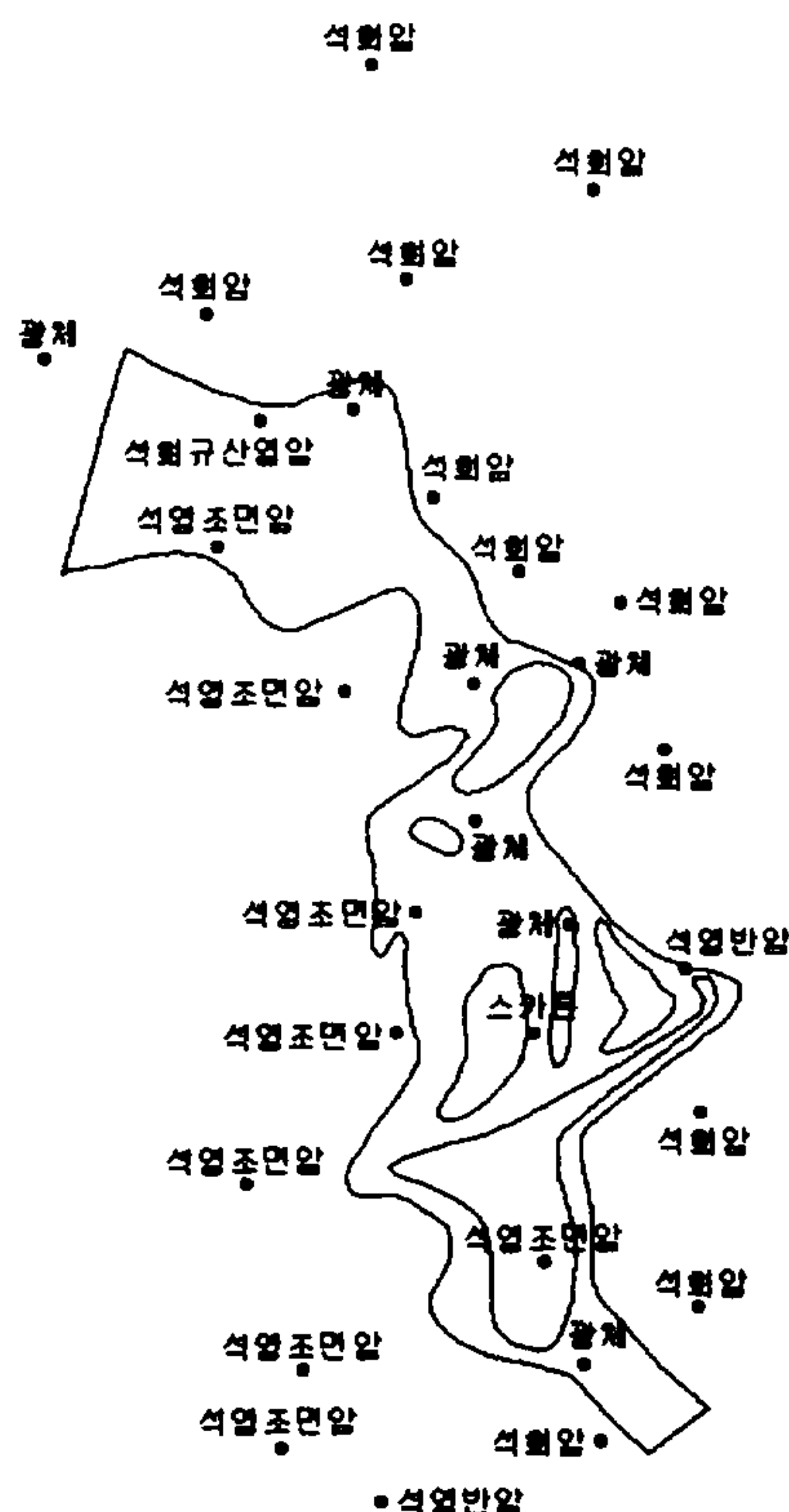
Fig. 23 The lithology of the cross-section obtained from the vertical and inclined well cores.
